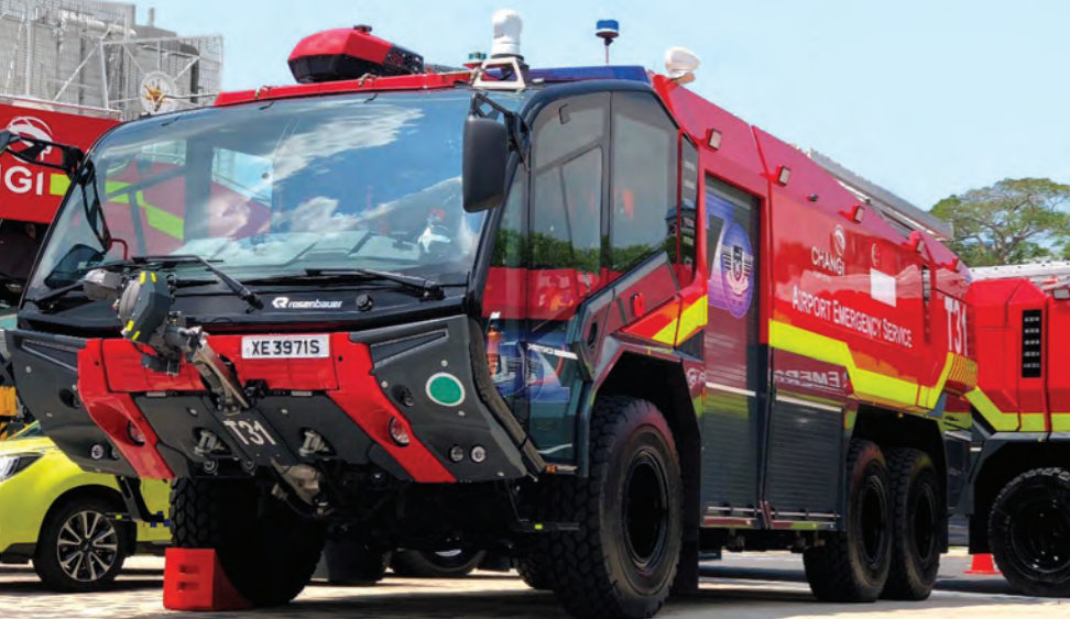
Bottom: The Rosenbauer Foam Tender can store up to 12,500 litres of water and 1,500 litres of foam.
